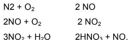
But this process requires high amount of electric power and high capital cost. It requires about five times as much electricity to fix a ton of N as is required by the cyanamide process. But this method is found to be suitable for countries like Scandinavia and Norway where the electricity is very cheap.
