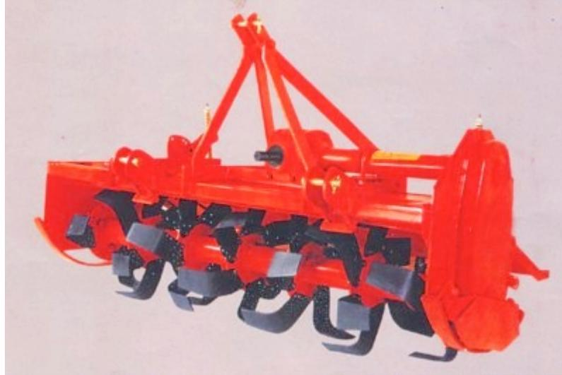
**Rotary tiller- Tractor operated**
