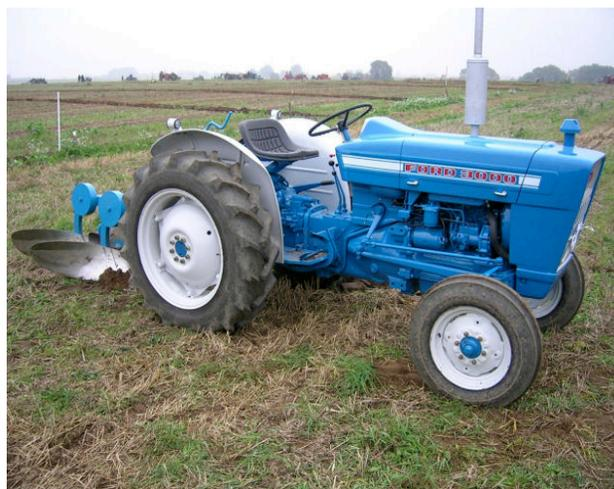
**Tractor with two bottom mouldboard plough**
