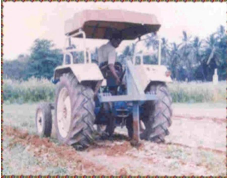
**Chisel plough in operation**
