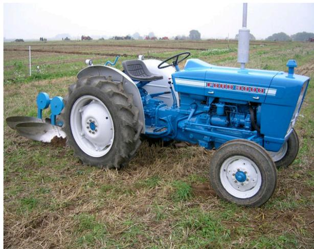
**Tractor with two bottom mouldboard plough**
