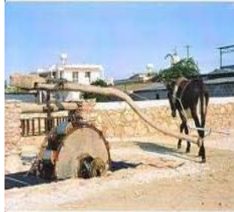
Persian wheel- water lifting
