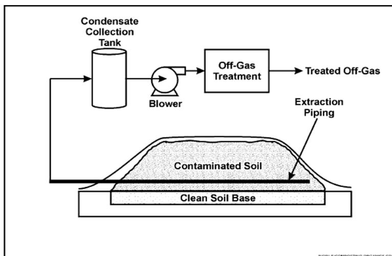
of surface contamination with petroleum hydrocarbons they are a refined version of landfarming that tend to control physical losses of the contaminants by
