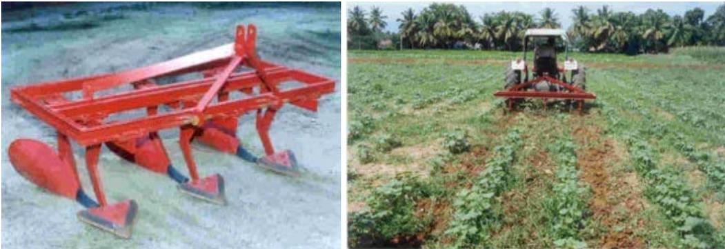
An inter cultivator cum earthing up equipment was developed and fitted to a standard tractor drawn ridger. Three number of sweep type blades are affixed to the ridger frame for accomplishing the weeding operation in between standing rows of crops. Three ridger bottom fitted behind the sweep blade, work on the loosened soil mass and aid in earthing up by forming ridges and furrows. Weeding efficiency is 61 per cent.
