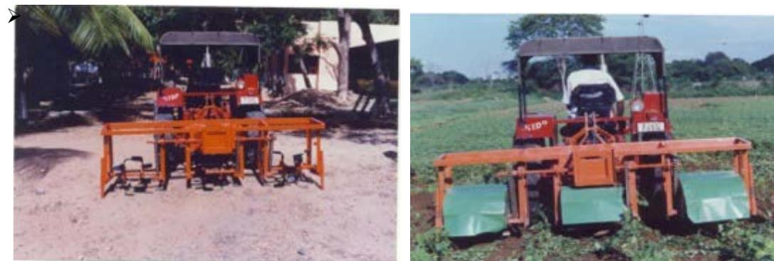
The multi row rotary weeder consists of a set of cutting blades, which penetrate in to the soil, removing the weeds in the crop rows. The cutting blade has also been used as an inclined plane for elevating and converging the soil. The rotating blades are used to cut the weeds and pulverizing the soil. Weeding efficiency is 71 per cent.
