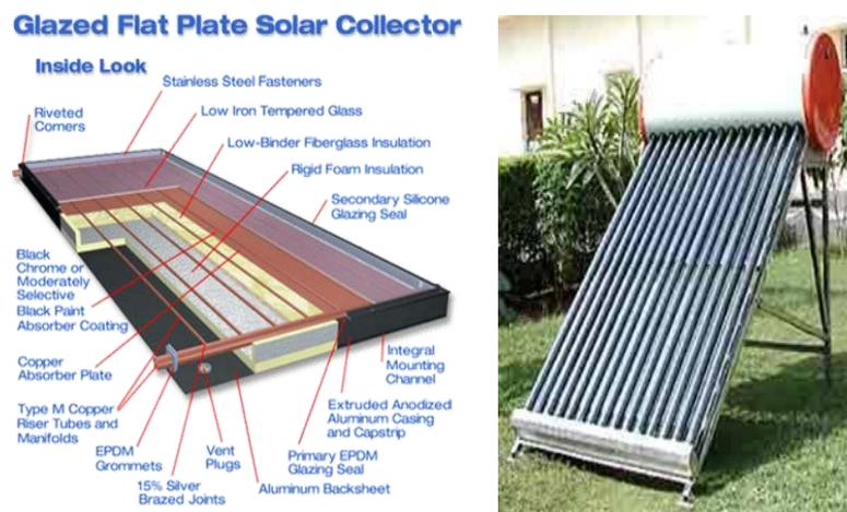
Fig.3 .Flat Plate liquid collector
